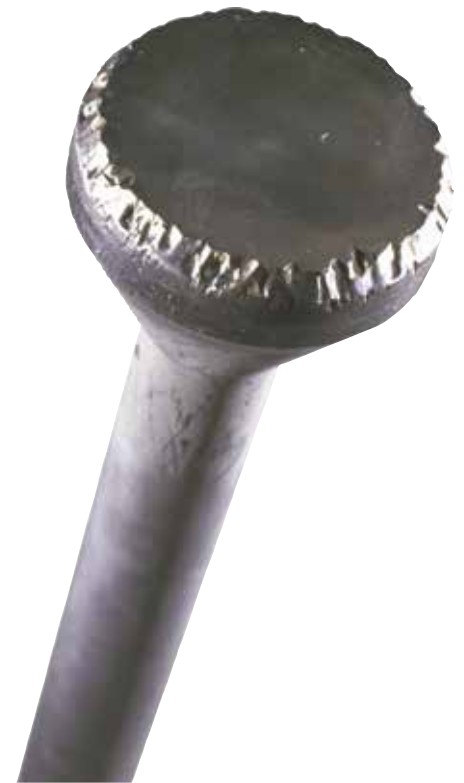
Erosion damage to a competitor’s valve plug caused by high fluid velocity results in poor shutoff.
