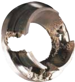
Seat ring damage caused by cavitation results in leakage that can harm downstream equipment.
